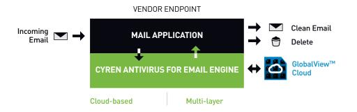
Spam classifications are provided to the engine from a local cache, or, if the email patterns are not identified locally, via a fast query to the GlobalView™ Cloud. The result is instant protection from new outbreaks without any lag in updates.
