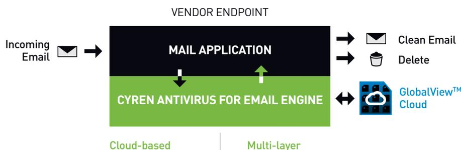
Spam classifications are provided to the engine from a local cache, or, if the email patterns are not identified locally, via a fast query to the GlobalView™ Cloud. The result is instant protection from new outbreaks without any lag in updates.
